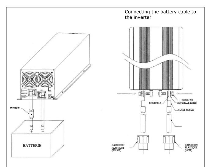
Do not place anything between the battery and the surface of the terminal. Assemble exactly as indicated in the diagram.
